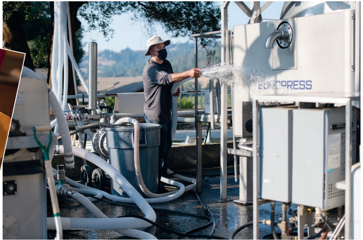
As with cooking, cleanup is half of the work of winemaking. We start cleaning after all the grapes have been destemmed and pressed for the day. A destemmer is on the left, a press is on the right—with a portable hot water generator tucked in below—and in the background an air-powered pump and a bucket of water accompany Alfredo, who is doing the hard work of cleaning.
